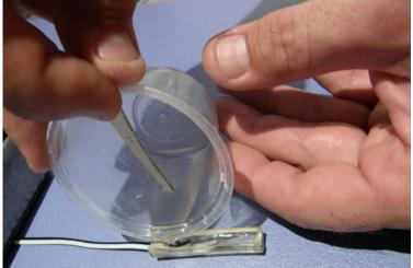
pouring resin into the mould containing the magnetic switch
