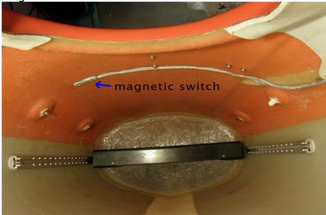
When the magnet and the switch are together the circuit will be closed (ON) and the electric bilge pump activated.
