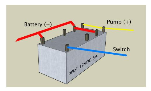
The best location for the relay is probably in the Pelican box next to the battery A wiring diagram for the whole system should be like this:
