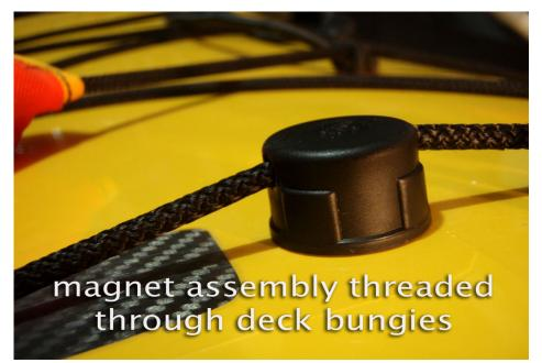
The magnetic switch will be positioned directly under the deck in the same position of the magnet above deck.
