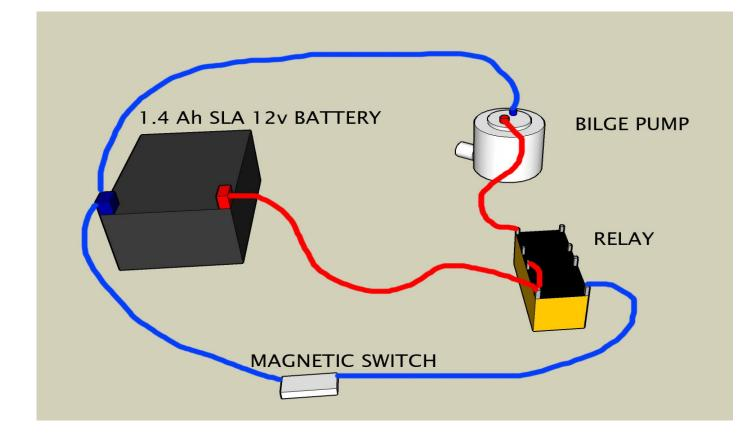
I have omitted the fuse between the battery and the bilge pump.
