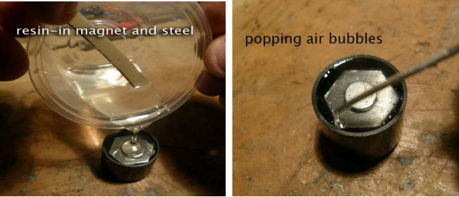
Remove any air bubbles with a pin.
