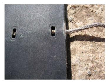
As you can see, the cable has been moulded into the plastic. I thought this might be game over, but I put the cable into a vice and started twisting - as if to unscrew the cable from the skeg. Fortunately they both came out like this. I'd recommend snugging the skeg right up against the vice before you start tightening - when I didn't do this the cable started to crack and fray and I thought it might just twist off.
