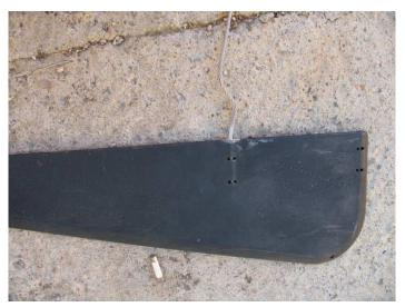
Then as with yours I got plenty glue into all the holes, and worked the cable through it a few times to get it all well coated, then left to harden.
