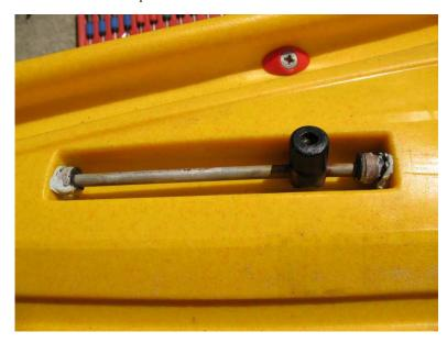
Removing the screw (philips head) allows the cable to be withdrawn. That is, if the head of the screw does not immediately shear out leaving a really tricky job to drill out 15mm of screw without destroying the plastic toggle! I opted to drill it all out a bit larger, then fill the void with araldite, and then drill out the araldite to the right size for a new screw....what a carry on!
