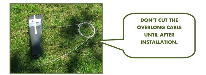
Here is the new skeg / cable assembly laid out on the moss and grass that pretends it's a lawn in my back garden. It's a long cable (2515mm / 8' 3"), but don't cut it until after installation unless you have proper BOWDEN CABLE cutters, like those used in bike shops. P&H provide a new grub screw and Allen key for other variants.
