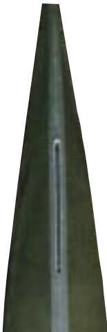
Keel Strip shown on translucent Kevlar/carbon hull
