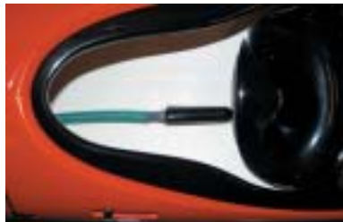
Strum box on the end of bilge pump pick-up hose
